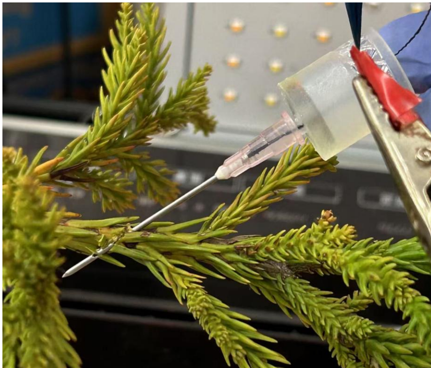
Figure S5. Photograph of needle type sucrose sensor inserted into Japanese cedar.
