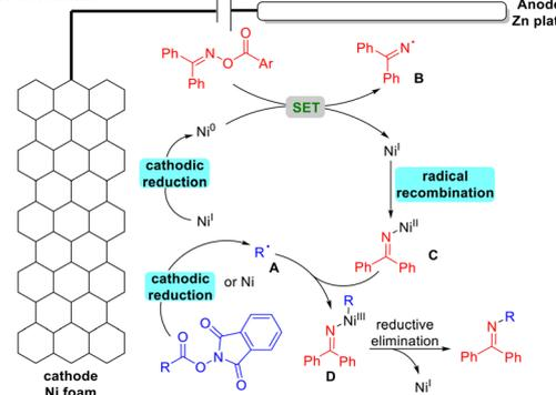
Scheme 18 Electrochemical Ni-catalyzed decarboxylative amination of NHPI esters.
