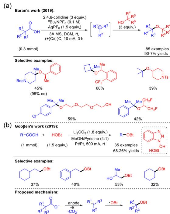
**Scheme 29** Electrochemical decarboxylative C(sp<sup>3</sup>)-O coupling reactions.
