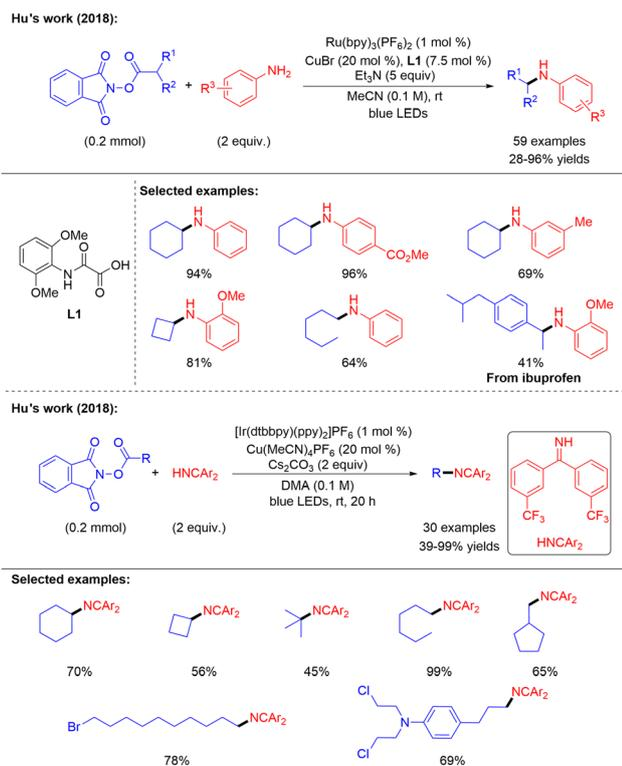
**Scheme 12** Synergetic photoredox and Cu-catalyzed C(sp<sup>3</sup>)-N decarboxylative amination.
