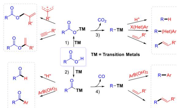
Scheme 1 Four common reaction types of carboxylic acids.
