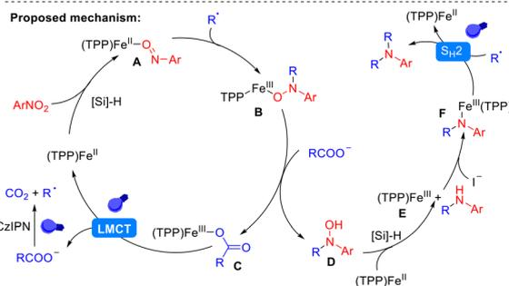
**Scheme 15** Synergetic photoredox and FeI<sub>2</sub>-catalyzed C–N decarboxylative amination.
