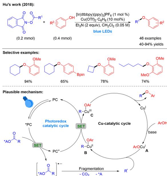
**Scheme 25** Synergetic photoredox-induced and copper-catalyzed decarboxylative alkoxylation.
