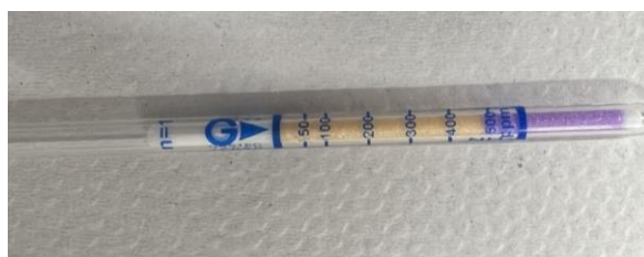
Fig. 5 Ammonia detection after the ball mill experiment.
