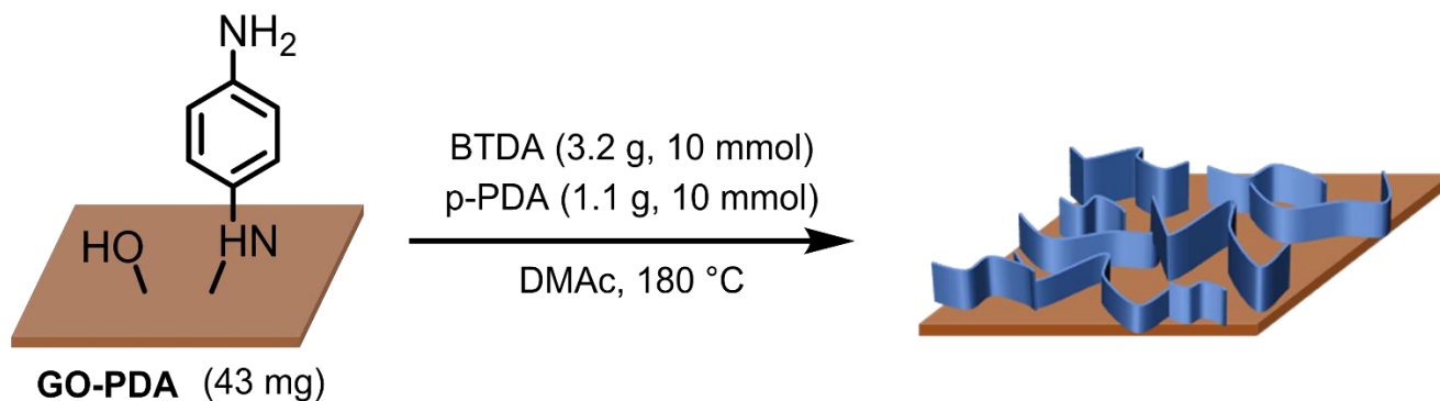
Fig. 6 Schematic illustration of the formation mechanism of PI-GO .
