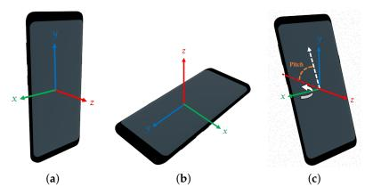
**Figure 2.** Gyroscope orientation on the smartphone. (a) position parallel to y-axis; (b) position parallel to x-axis; (c) position of the pitch.
