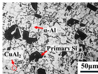
Figure 3. Optical micrograph showing microstructure of GC sample.
