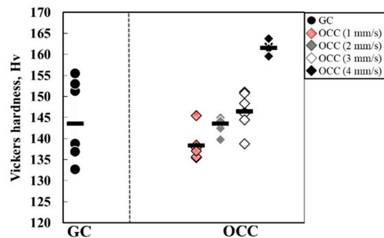
Figure 9. Vickers hardness of GC and OCC samples.
