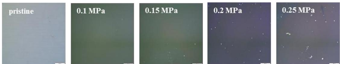
Figure 4.4: Digital micrographs of HNO<sub>3</sub> treated PEDOT:PSS films showing the surface conditions at various pressures of N<sub>2</sub> gas. The scale bars in all photos are 500  $\mu\text{m}$ . All photos were captured at a magnification of 7.5X.
