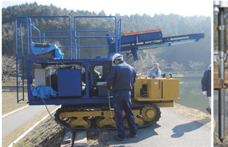
Fig. 2.3 Cone penetration machine and attached cone
