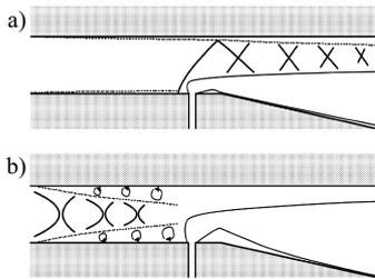
Fig. 5. Schematic flow image of combustors in (a) scramjet mode operation and (b) dual-mode operation.
