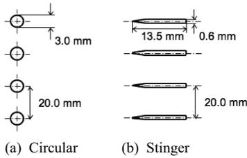
Fig. 2. Schematic diagram of multi-injection orifices: (a) circular and (b) stinger shape. Fuel is injected in the direction perpendicular to the paper, while crossflow air travels left to right.
