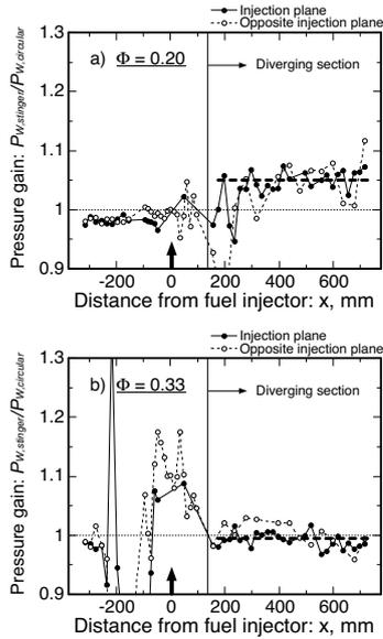
Fig. 4. Pressure gain with multiple stinger injectors at (a)  $\Phi = 0.20$  and (b)  $\Phi = 0.33$ .
