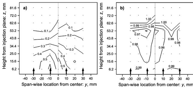
Fig. 7. Distributions of (a) local equivalence ratio and (b) combustion efficiency at the exit of the combustor with multiple circular injectors (left) and multiple stinger injectors (right) at  $\Phi = 0.33$ .
