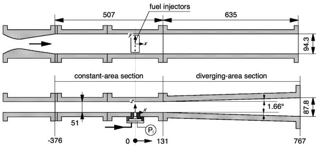
Fig. 1. Schematic diagram of supersonic combustor.
