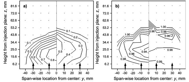
Fig. 6. Distributions of (a) local equivalence ratio and (b) combustion efficiency at the exit of the combustor with multiple circular injectors (left) and multiple stinger injectors (right) at  $\Phi = 0.20$ .
