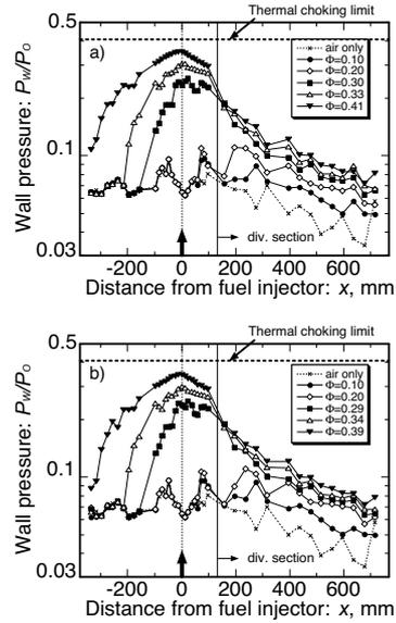
Fig. 3. Wall pressure distributions using (a) multiple circular injectors and (b) multiple stinger injectors at various  $\Phi$ .
