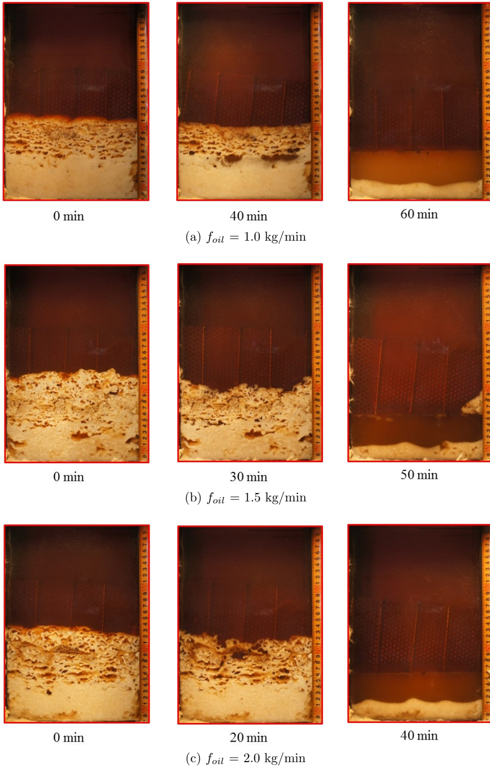
Figure 5.27: Melting behaviors of PCM with the perforated partition plate at the three types of oil flow rates.
