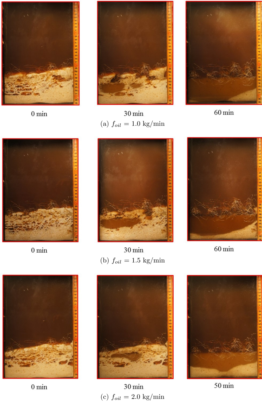
Figure 5.44: Melting behaviors of PCM with the metal fiber \phi = 0.5\% at the three types of oil flow rates.
