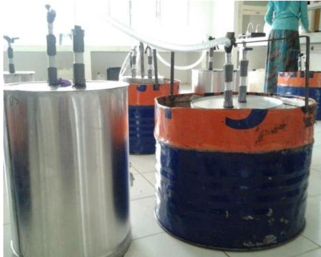
**FIGURE 1.** Biogas digester
