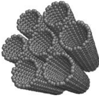
Figure 1-7. Van Der Wall interaction between SWCNTs leads to the formation of a bundle.
