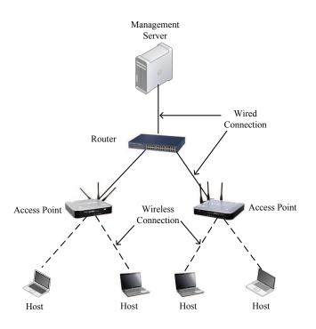
Figure 3.1: Example elastic WLAN system topology.
