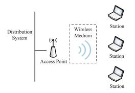
Figure 2.1: Components of WLAN system.
