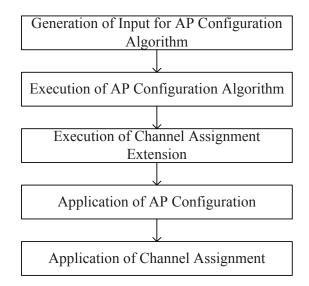
Figure 3.2: Operational flow of elastic WLAN system.
