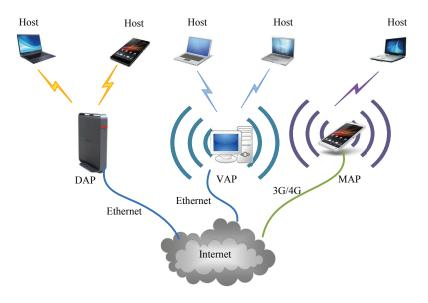
Figure 1.1: Illustration of elastic WLAN with heterogeneous devices.
