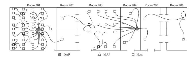
Figure 6.2: Solution for bandwidth limitation with mobile data plans scenario with H = 60, G = 5, data plan = 24*Mbps*, DAP=2, and MAP=8 in Kabi Nazrul University instance.
