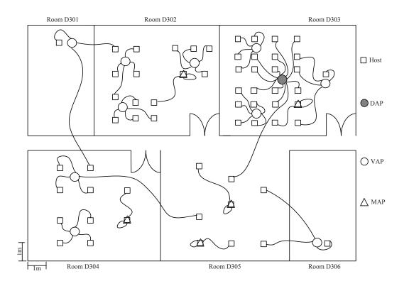
Figure 6.1: Solution of proposed algorithm for scenario with H = 60, G = 10, DAP=1, VAP=10, MAP=5, and data plan=30Mbps in Okayama University instance.
