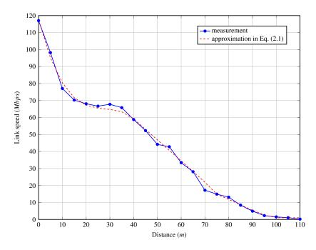
Figure 2.4: IEEE 802.11n link speed measurement results.
