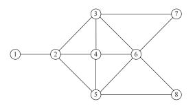
Figure 5.3: Interference graph of example channel assignment topology.
