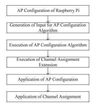
Figure 7.2: Elastic WLAN system execution flow.
