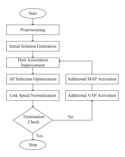
Figure 4.2: Flow chart of the AP configuration algorithm
