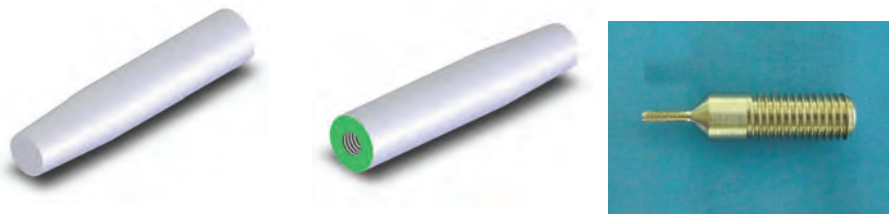
Fig. 2 The shape of the implants. Based on CT of rabbit femurs performed three times before implantation, the most suitable implant size was 4.8 mm dia. × 30 mm. Each implant was cylinder-shaped and hollow at one end so that a hook could be inserted to perform the pull-out test.
