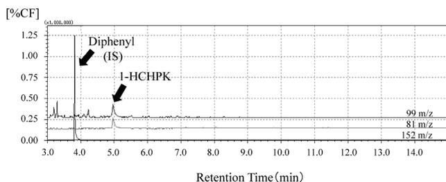
Fig. 2. GC-MS Chromatograms of Extracts from 20mL Vials of Water for Injection Solution
