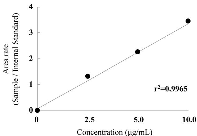
Fig. 3. Calibration Curve of 1-HCHPK
