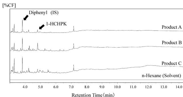
Fig. 1. GC Chromatograms of Extracts from 20mL Vials of Water for Injection Solution
