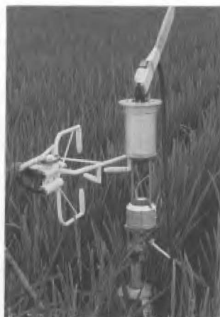
Photo 1 Installation of infrared \text{CO}_2 \text{H}_2\text{O} fluctuation meter and sonic anemometer thermometer assembly above a paddy field
