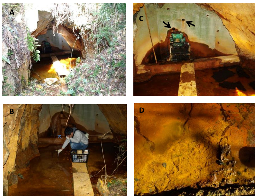
Fig. 2-3. Photographs of a sampling site (Yasumi-ishi tunnel). A, Yasumi-ishi tunnel; B, ARD seeps through the hole of tunnel. Precipitates of iron hydroxides are formed in the pond.; C, arrows indicate the hole from which ARD sample for an analysis of physicochemical properties was collected; D, RAD-containing sediments were collected to analyze microbial community structure.
