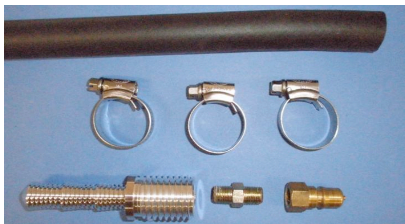
Fig. 3.17 Parts of high hydraulic artificial muscle
