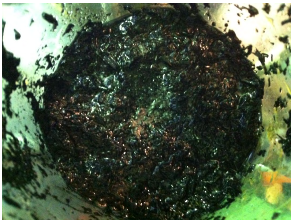
A 41—Picture of the charcoal in the column after the experiment was stopped (2). The charcoal were taken out in 2-3 cm layers and the total iron content was measured.
