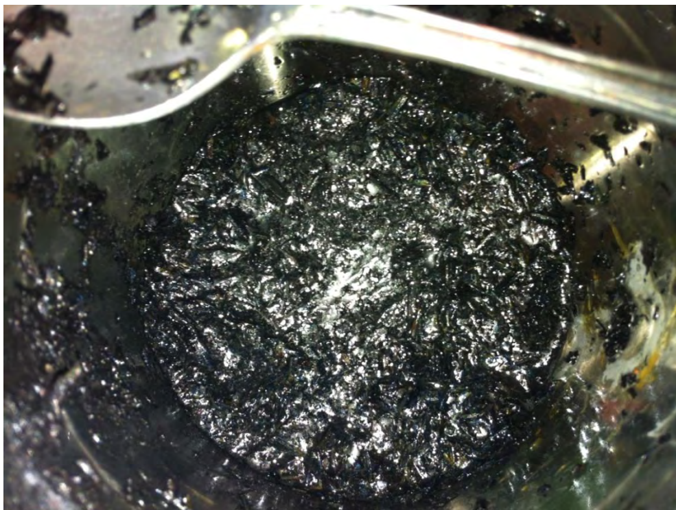
A 40—Picture of the charcoal in the column after the experiment was stopped (1). The charcoal were taken out in 2-3 cm layers and the total iron content was measured.
