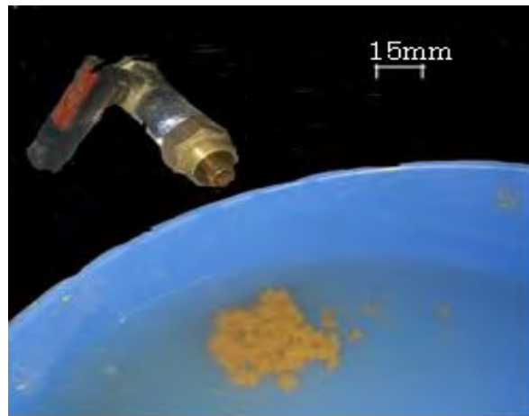
Figure 3.19—Picture of the outflowing iron precipitates during back flushing.
