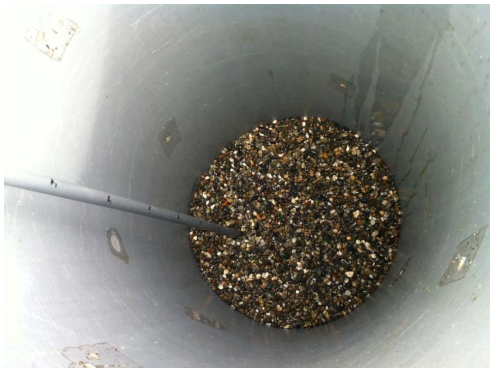
A 48—Gravel layer at the bottom of the charcoal filter at the field site.
