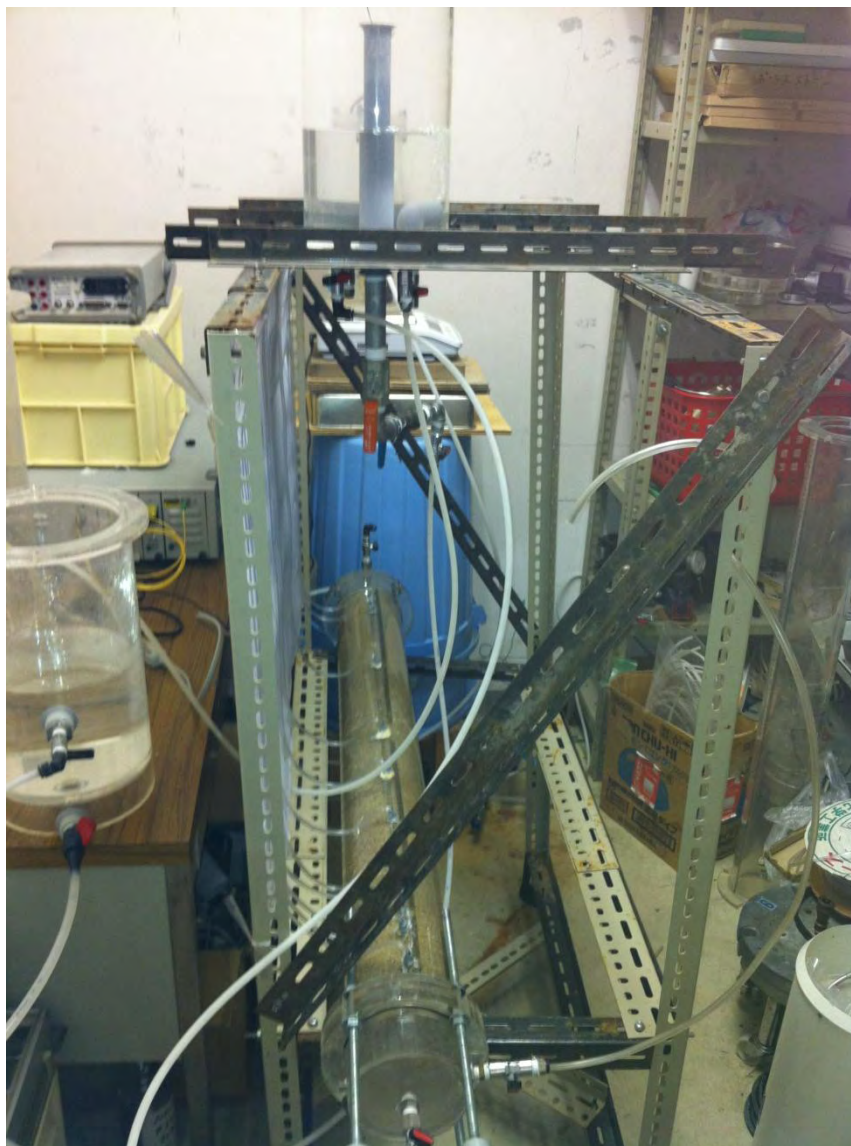
A 39—Experimental setup of the one-dimensional particle mobilization experiment regarding physical clogging in the laboratory.
