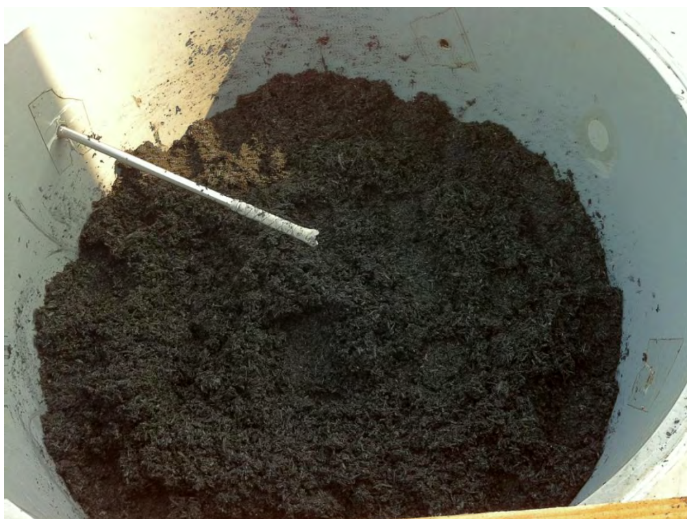
A 51—Picture of filling the charcoal into the filter column. It is also one sampling port shown, reaching to the middle of the column.
