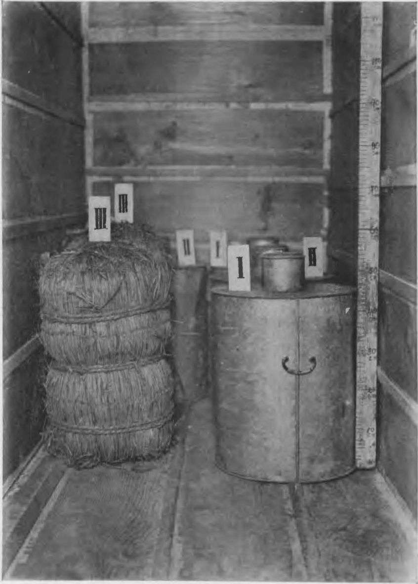
Storage of the hulled rice in the granary of the Ōhara Institute. I. Air-tight storage in the zinc vessels. II. Carbon dioxide storage in the zinc vessels. III. Straw-bags storage.
