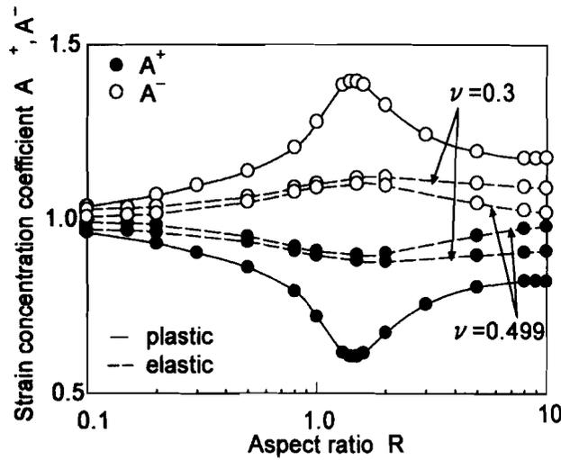
Fig. 5 Relation between strain concentration coefficients and aspect ratio for three-dimensional rigid-plastic and elastic deformations [  $\phi = 0.2$  ]
