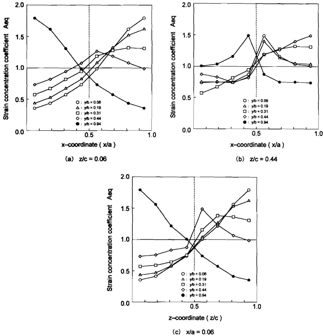
Fig. 2. Distribution of strain concentration coefficient  $A_{eq}$  in Model A
