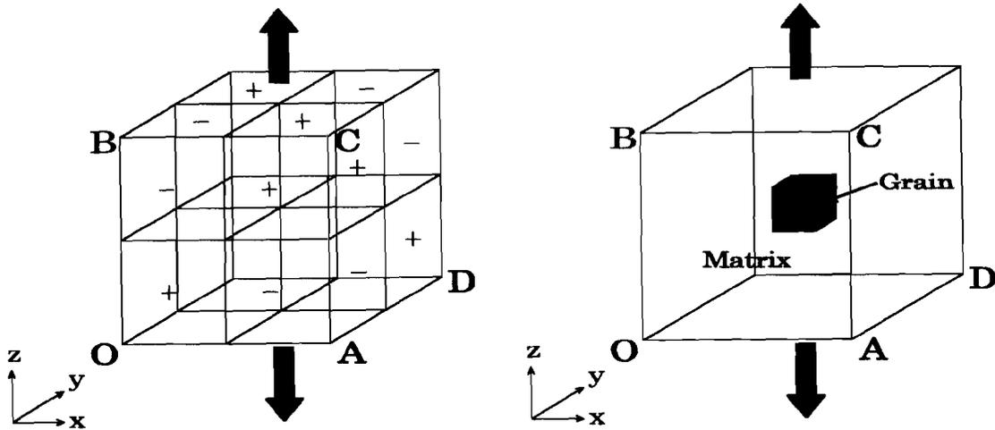
(a) Model A: regularly placed grains (b) Model B: grain imbedded in matrix
