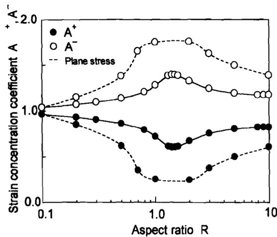
Fig. 4. Relation between averaged strain concentration coefficients  $A^+, A^-$  and aspect ratio  $R$  ( $\phi = 0.2$ )
