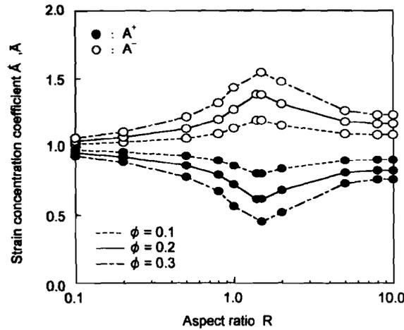
Fig. 3 Relation between averaged strain concentration coefficients  $A^+, A^-$  and aspect ratio  $R$
