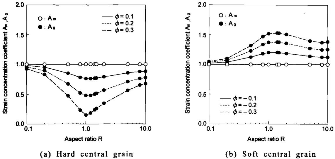
Fig. 6 Relation between averaged strain concentration and aspect ratio
