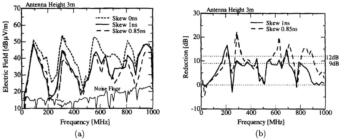
Figure 13: The measurement results of far electric field at an antenna height of 3 m. (a) The spectrum of electric field. (b) The amount of reduction.
