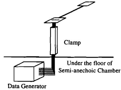
Figure 10: Connection of the generator and the board.
