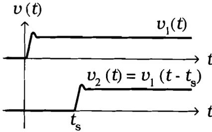
Figure 1: Waveforms with skew between channels (2 lines).
