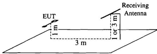
Figure 9: The location of EUT and the antenna in the far electric field measurement.
