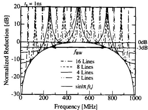
Figure 6: The amount of normalization reduction of a synthetic voltage spectrum.
