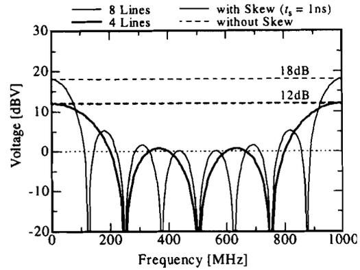
Figure 4: The synthetic voltage spectrum of many lines.
