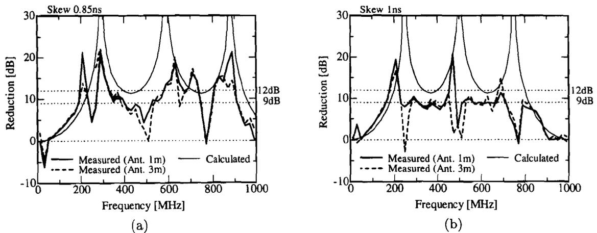
Figure 14: The measurement and calculation result of the amount of far electric field reduction (a) skew 0.85 ns and (b) skew 1 ns.
