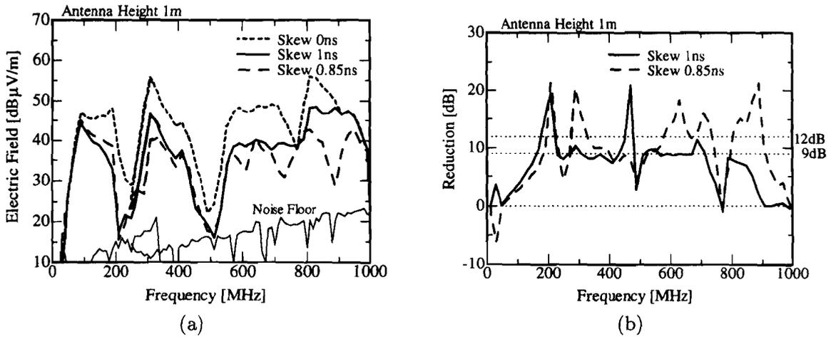
Figure 12: The measurement results of far electric field at an antenna height of 1 m. (a) The spectrum of electric field. (b) The amount of reduction.
