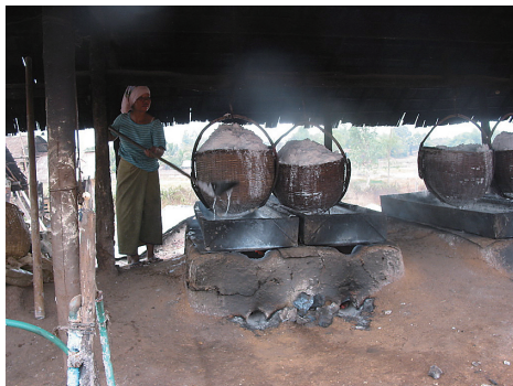
Fig. 24 Salt from underground water (2004, Laos)
