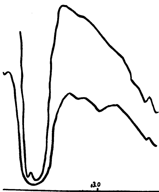
Fig. 3. Infra-red absorption spectrum of monoether around 3\mu .
