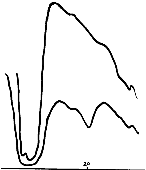
Fig. 2. Infra-red absorption spectrum of dilirubin-dimethylester around 3\mu .
