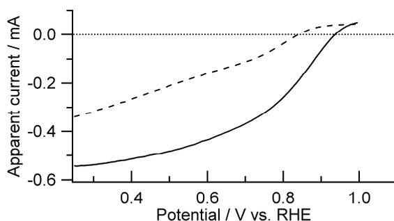
**Fig. 4** Hydrodynamic voltammograms at 900 rpm under an oxygen atmosphere of Pt-GO heated at 673 K in air (solid line) and Pd-GO heated at 673 K in N<sub>2</sub> (broken line).
