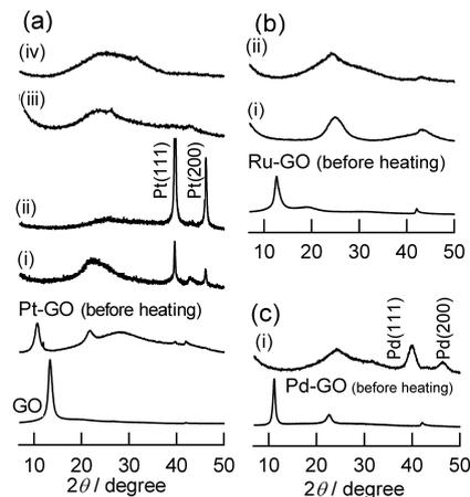
**Fig. 2** X-ray diffraction (XRD) patterns of raw materials and heated samples: (a) GO and Pt-GO (before heat treatment), and the latter Pt-GO heated at 573 K (i), 673 K (ii) in air, 573 K (iii), 673 K (iv) in N<sub>2</sub>; (b) Ru-GO (before heat treatment) and Ru-GO heated at 573 K (i), 673 K (ii) in N<sub>2</sub>; (c) Pd-GO (before heat treatment) and Pd-GO heated at 673 K (i).
