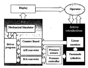
Figure 6. Block diagram of active link mechanism system
