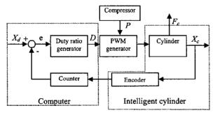
Figure 11. Control system of intelligent cylinder
