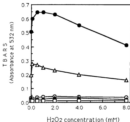
**Fig. 7** The effects of  $H_2O_2$  addition on TBARS generation from liposomes by FeNTA- or CuNTA-induced lipid peroxidation. Liposomes were incubated for 60 min in the presence of various concentrations of  $H_2O_2$  with (●) 2 mM FeNTA and 2 mM ascorbate, (○) 2 mM FeNTA, (▲) 2 mM CuNTA and 2 mM ascorbate, (△) 2 mM CuNTA, and (□) liposomes alone.
