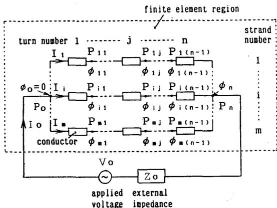
Fig.3 Equivalent circuit of winding.
