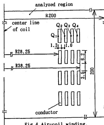
Fig.4 Air-coil winding.
