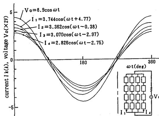
Fig.5 Time variations of applied voltage and currents.
