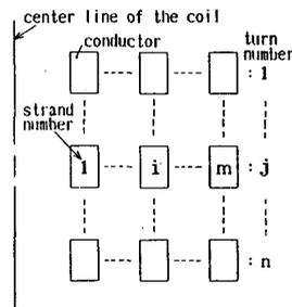
Fig.2 Cylindrical winding with multi-conductors.
