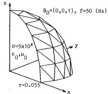
Fig. 7 A conducting sphere model.
