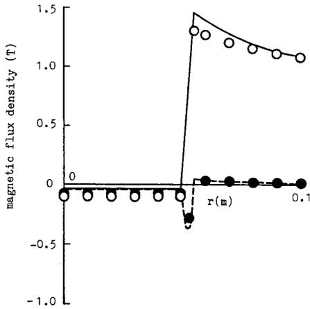
Fig. 4 Distributions of magnetic flux density in the hollow sphere, on x-y plane.
