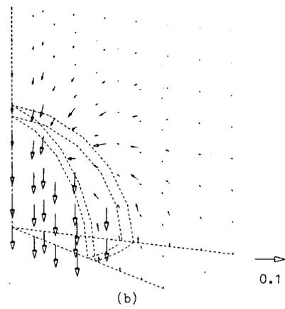
Fig. 6 Distributions of magnetic flux density vectors in the hollow sphere model, (a) real part, (b) imaginary part.
