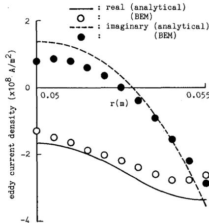
Fig. 3 Distributions of eddy current density in the hollow sphere, on x-y plane.
