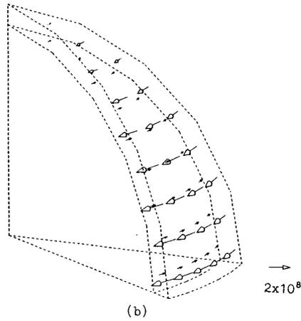
Fig. 5 Distributions of eddy current density vectors in the hollow sphere, (a) real part, (b) imaginary part.
