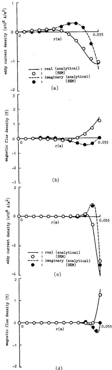
Fig. 8 Distributions of eddy current density and magnetic flux density in the sphere model on x-y plane, (a) eddy current density,  $f=50 \text{ Hz}$ , (b) magnetic flux density,  $f=50 \text{ Hz}$ , (c) eddy current density,  $f=500 \text{ Hz}$ , (d) magnetic flux density,  $f=500 \text{ Hz}$ .
