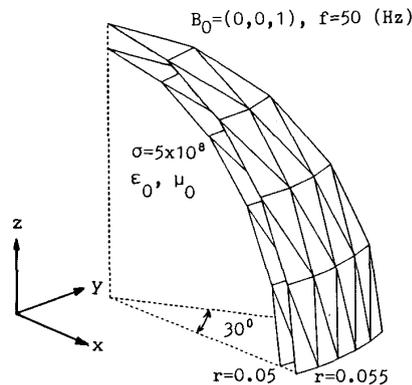
Fig. 2 A conducting hollow sphere model.
