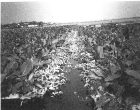
Fig.6 Photograph of experiment on water cleaning by plants floating culture system in L.Wuli.
