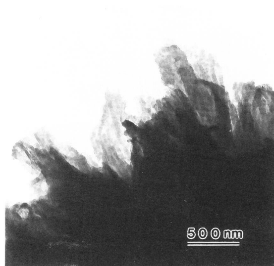
Fig.5 Electron micrograph of cis-PBZT crystal prepared by slow cooling from 110 °C to room temperature in 92wt% H 2 SO 4
