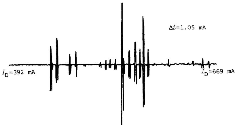
Fig.9 Trace of 2f spectrum of methane, 3 Torr, 100%.
