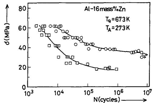
Fig.8 S-N curves of the 16%Zn alloy aged at 273K after quenching from 673K. Thickness of the surface layer removed: ○ 0 μm, □ 50 μm.
