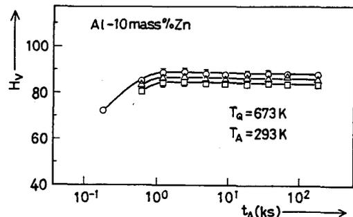
Fig.2 Position dependence of the age-hardening curve.  $\circ$  far from the grain boundary(GB),  $\Delta$  near the GB,  $\square$  on the GB.
