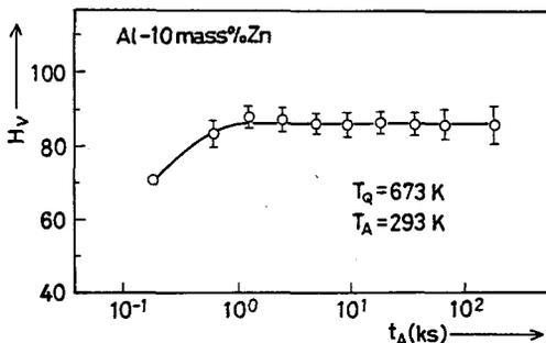
Fig.1 Age-hardening curve of the 10%Zn alloy at 293K after quenching from 673K.
