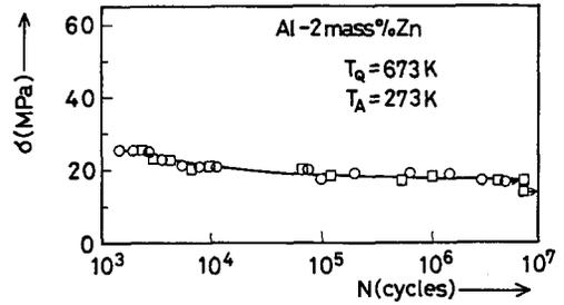
Fig.6 S-N curve of the annealed 2%Zn alloy. Thickness of the surface layer removed: ○ 0 μm, □ 50 μm.
