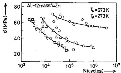
Fig.4 S-N curves of the aged 12%Zn alloy. Thickness of the surface layer removed:  $\circ$   $0\mu\text{m}$ ,  $\triangle$   $10\mu\text{m}$ ,  $\square$   $50\mu\text{m}$ ,  $\nabla$   $100\mu\text{m}$ .
