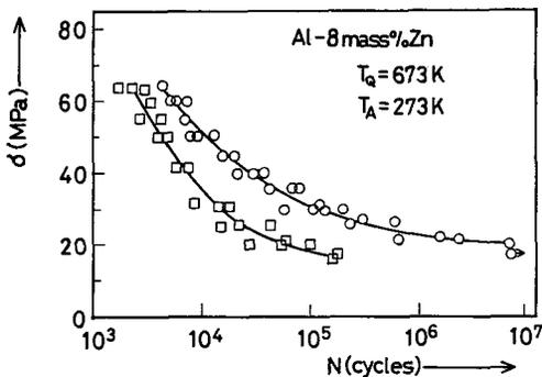
Fig.7 S-N curves of the 8%Zn alloy aged at 273K after quenching from 673K. Thickness of the surface layer removed: ○ 0 μm, □ 50 μm.
