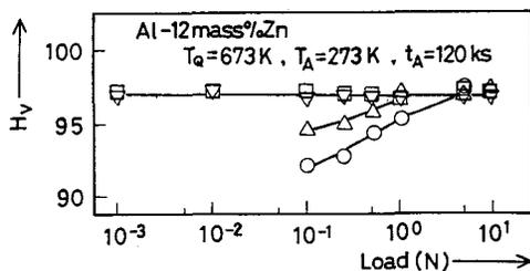
Fig.3 Hardness vs. load plot of the 12%Zn alloy aged at 273K for 120ks after quenching from 673K. Thickness of the surface layer removed by electropolishing is  $\circ$   $0\mu\text{m}$ ,  $\triangle$   $50\mu\text{m}$ ,  $\square$   $100\mu\text{m}$ ,  $\nabla$   $150\mu\text{m}$ .
