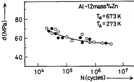
Fig.5 Effect of the surface polishing on the S-N curve of the aged 12% alloy. ○ non-electropolished, ● electropolished before aging.
