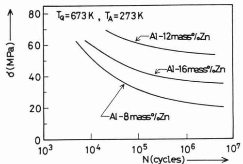
Fig.9 Variation of the S-N curves of the aged Al-Zn alloy with composition.
