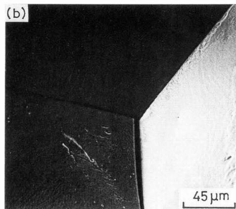
SEM fractographs of fatigue failure: (a) 8%Zn alloy, (b) 16%Zn alloy.
