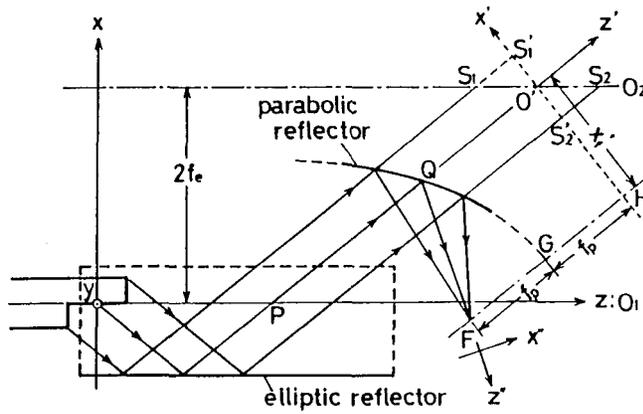
Fig. 8 Beam focusing by a parabolic cylinder reflector.
