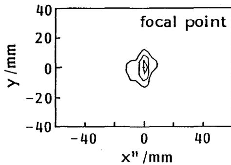
Fig. 13 Measured power distributions around the focal point focused by two cylindrical reflectors; equipower contours at levels of 0.75, 0.5 and 0.25.
