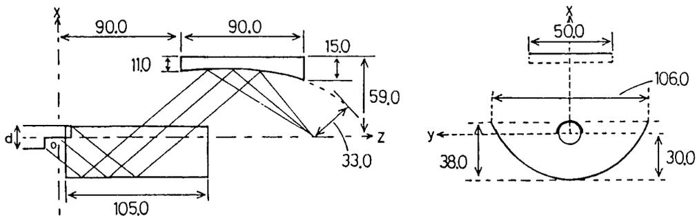
Fig. 10 Dimensions of the experimental antenna.
