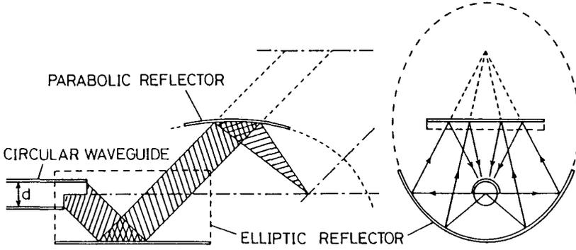
Fig. 2 Beam focusing antenna for  $TE_{0n}$  mode.
