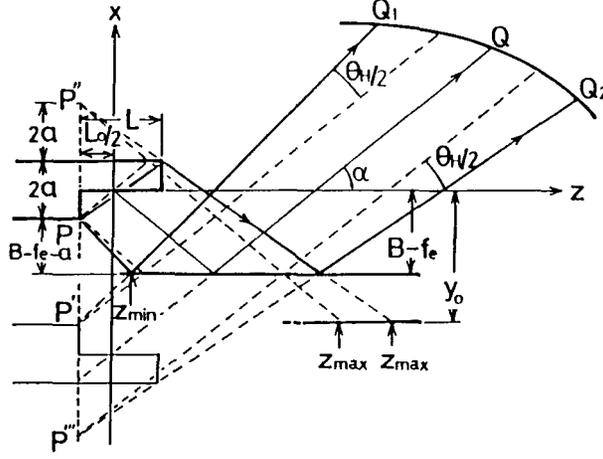
Fig. 7 Required dimensions of the reflectors in consideration of diffraction.
