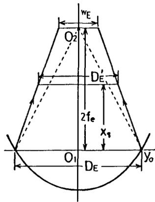
Fig. 9 Determination of the width of the second reflector: half-power width  $w_E$ ; the width of the parabolic reflector  $D'_E$ ; the width of the elliptic reflector  $D_E$ .
