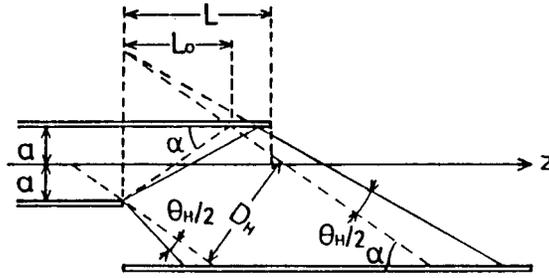
Fig. 3 Required length of the semicircular visor.
