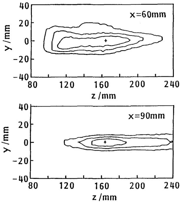
Fig. 12 Measured power distribution on the planes parallel with the  $yz$ -plane focused by an elliptic cylinder reflector only; equipower contours at levels of 0.75, 0.5 and 0.25.
