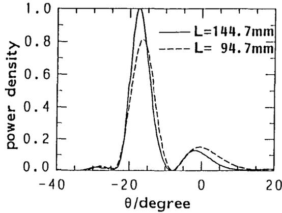
Fig. 4 Measured radiation pattern from circular waveguides with different length of semicircular visors: TE<sub>01</sub> mode; waveguide radius  $a = 16$  mm; frequency  $f = 35.5$  GHz;  $\alpha = 18.8^\circ$ ;  $L_o = 94.1$  mm.
