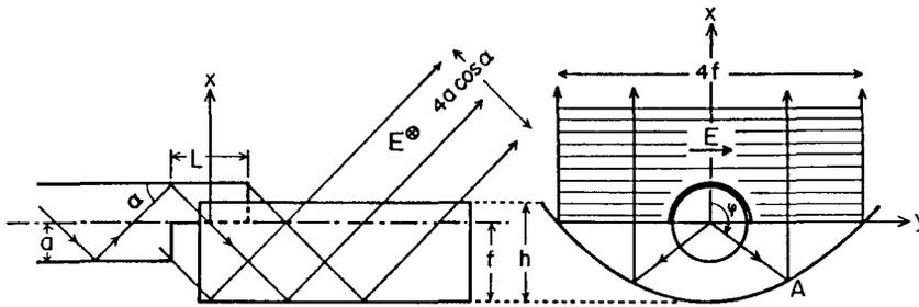
Fig. 1 Quasi-optical antenna having a parabolic cylinder reflector.
