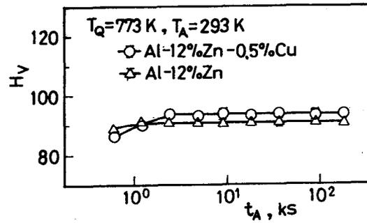
Fig.3 Isothermal age-hardening curves of the Al-12 mass%Zn binary alloy and Cu-added alloy aged at 293K after quenching from 773K.
