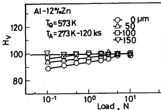
Fig.4 Dependence of hardness on the indentation load for the binary alloy specimen just aged at 273K for 120ks after quenching from 573K and the ones aged and electropolished to remove the surface layers.
