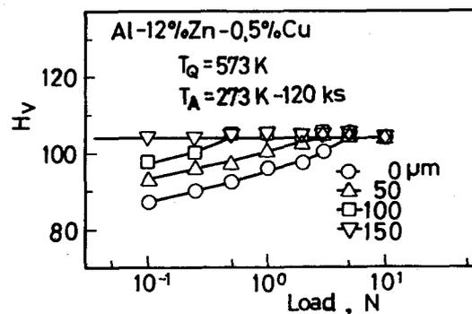
Fig.5 Dependence of hardness on the indentation load for the Cu-added alloy specimen just aged at 273K for 120ks after quenching from 573K and the ones aged and electropolished to remove the surface layers.
