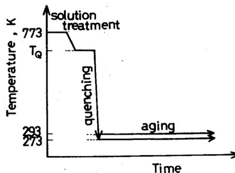
Fig. 1 Schematic diagram of the sequence of heat treatment.
