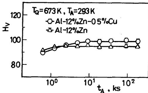
Fig.2 Isothermal age hardening curves of the Al-12 mass%Zn binary alloy and Cu-added alloy aged at 293K after quenching from 673K.
