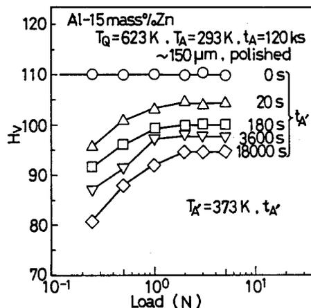
Fig.8 Dependence of hardness on the load at several stages of isothermal annealing of Fig.7. ○ 0s, △ 20s, □ 180s, ▽ 3600s, ◇ 18000s.
