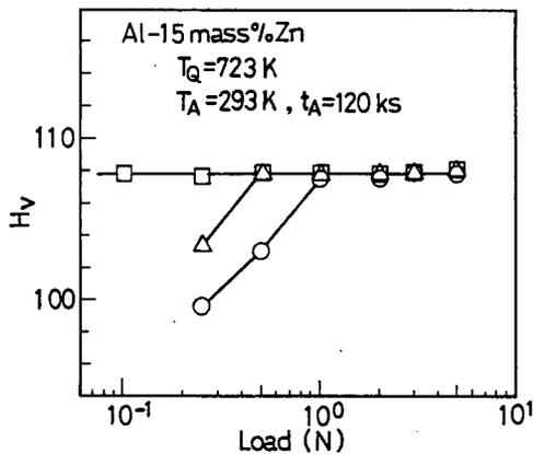
Fig.1 Variation with the thickness of surface layer removed, of the dependence of hardness on the indentation load, for the specimen aged for 120ks at 293K after quenching from 723K. Removed thickness:  $\circ$   $0\ \mu\text{m}$ ,  $\triangle$   $30\ \mu\text{m}$ ,  $\square$   $75\ \mu\text{m}$ .
