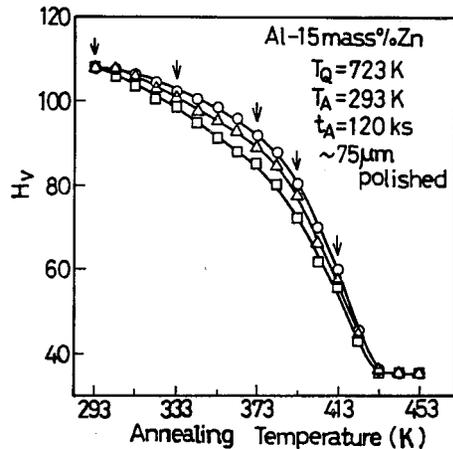
Fig.2 Variation of the isochronal annealing curve with the position of indentation for the specimen aged as in Fig.1 and electropolished to remove  $75\ \mu\text{m}$  thickness of surface layer. Indentation load was  $0.49\text{N}$ .  $\circ$  far from GB,  $\triangle$  near GB,  $\square$  on GB.
