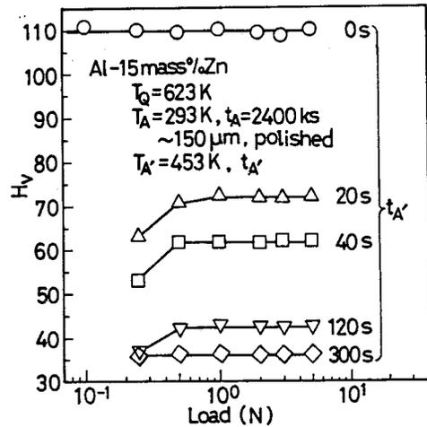
Fig.10 As Fig.8, but for the annealing temperature 453K.
