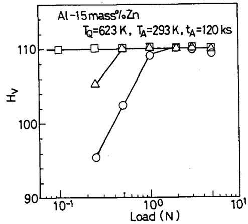
Fig.4 As Fig.1, but for the specimen aged after quenching from 623K.
