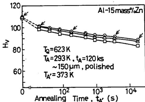
Fig.7 Isothermal annealing curves at 373K for the specimen aged after quenching from 623K and electropolished.
