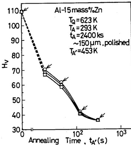
Fig.9 As Fig.7, but for the annealing temperature 453K.
