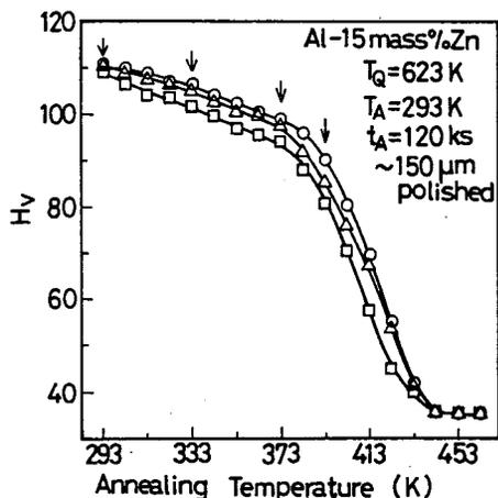
Fig.5 As Fig.2, but for the specimen aged after quenching from 623K.
