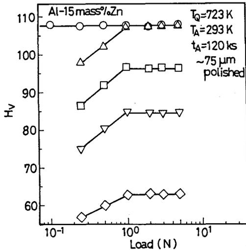
Fig.3 Dependence of hardness at position far from GB on the indentation load at several stages of isochronal annealing (marked by arrows in Fig.2).
