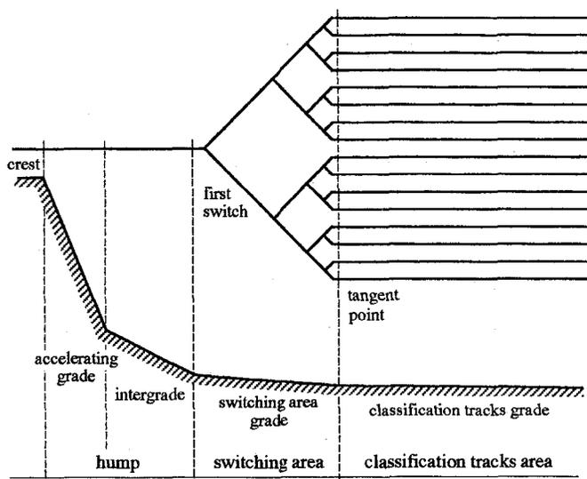
Figure 3: Horizontal and vertical layouts of the hump yard
