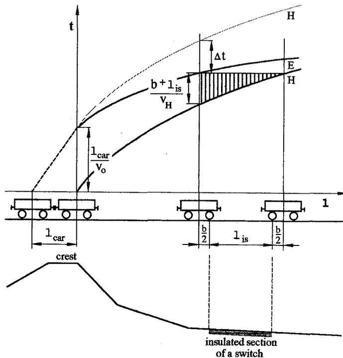
Figure 4: Spacing between cars in the switching area
