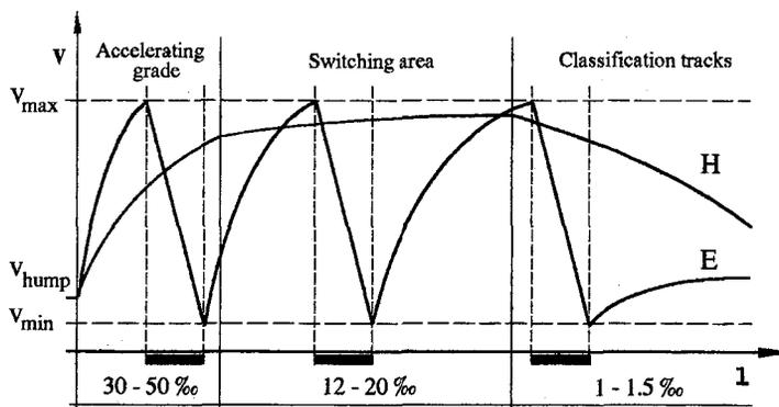
Figure 6: Velocity based placement of the retarders
