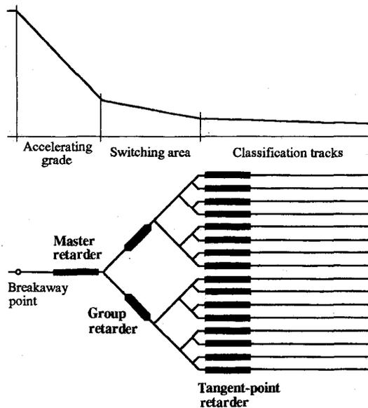
Figure 7: Placement of the retarders into the hump track formation
