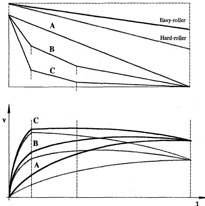
Figure 1: Car velocity as a function of the hump profile
