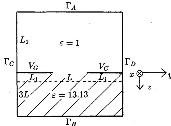
Figure 1: Model of two-dimensional split-gate quantum wire. In  $z$ -direction, electrons are confined by band offset in a plane shown by dotted line.
