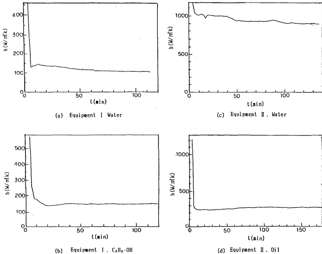
Fig.7 Heat transfer coefficient along the time proceeding
