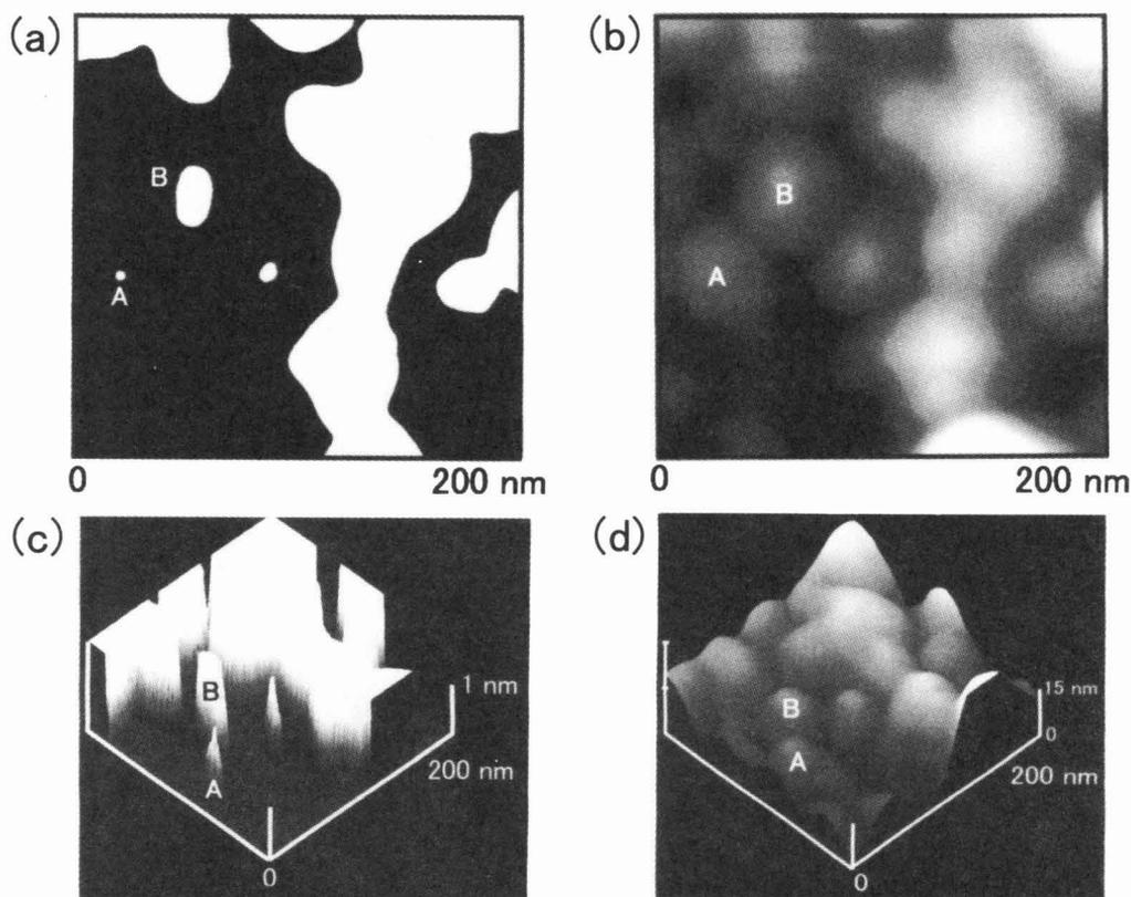
**Fig.5** SPM height image of rigid cilia of different length on a PBZT lamellar crystal observed (a) by direct RMS mode, (b) by the ordinary tapping mode. The contrast covers height variations in the 0 – 2 nm in (a) and in the 0 – 30 nm range in (b). (c) and (d) are bird's-eye views of (a) and (b) respectively.
