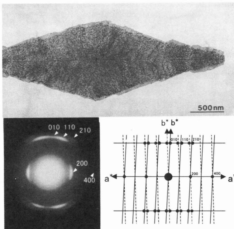
**Fig.1** TEM of lozenge PBZT lamellar crystal and its SAED with reciprocal lattice.
