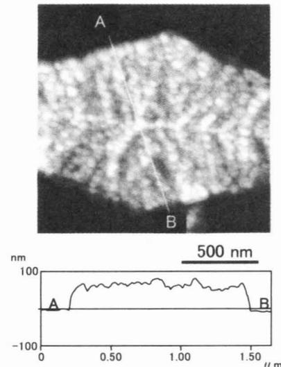
**Fig.2** SPM height image of PBZT lamellar crystal surface taken in the ordinary tapping mode. The cross-sectional height profile along the line A-B is shown below the image.
