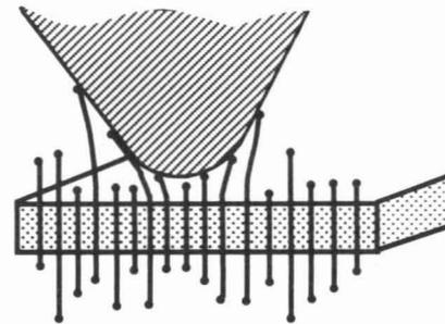
**Fig.3** Schematic illustration of rigid chains deformed by the tip of the cantilever during observation by the ordinary tapping mode
