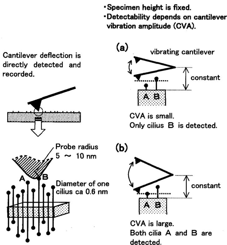
Fig.4 Schematic illustration of geometry between the amplitude of cantilever vibration and cilia on PBZT lamella
