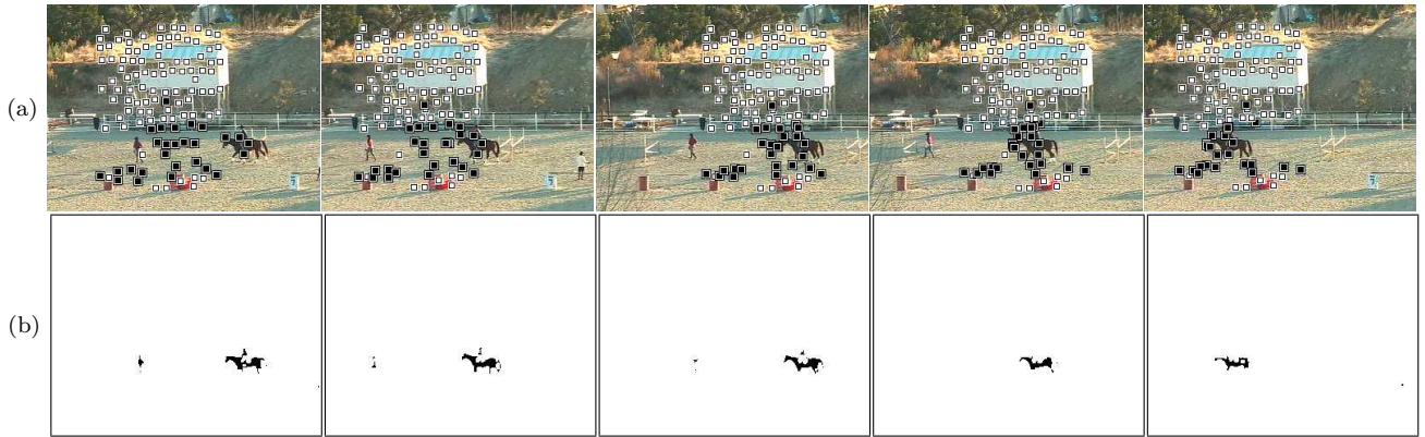
Figure 3: Five decimated frames from a 100 frame sequence (above) and detected moving objects (below).
