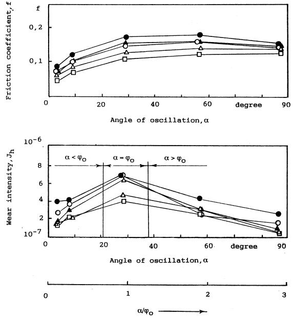
SLC: MoS<sub>2</sub>+epoxy resin ( $h=25\mu\text{m}$ )
