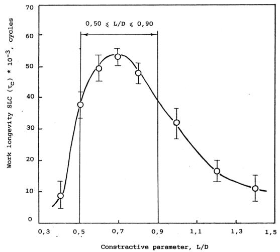
SLC: MoS<sub>2</sub>+epoxy resin ( $h=25\mu\text{m}$ )
