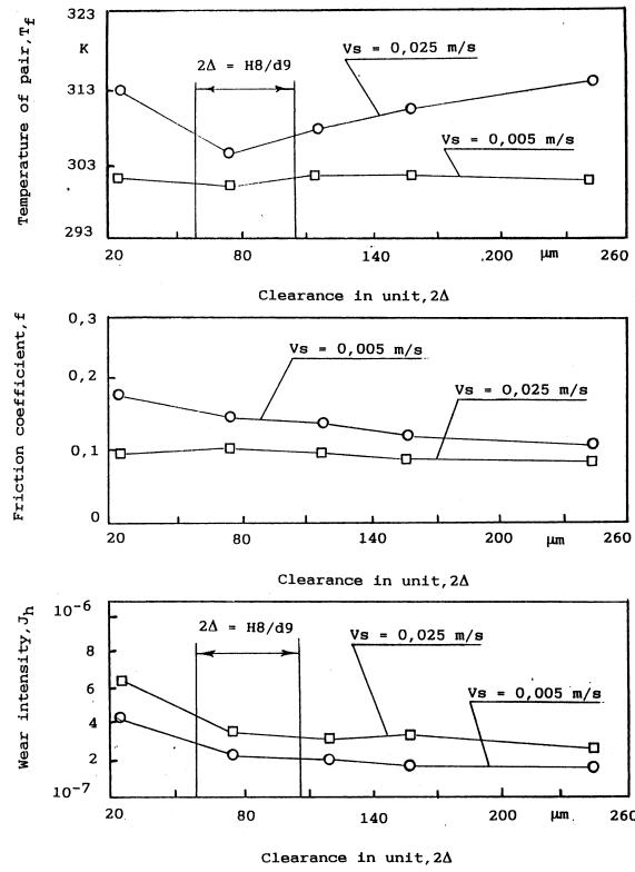
SLC: MoS<sub>2</sub>+epoxy resin ( $h=25\mu\text{m}$ )
