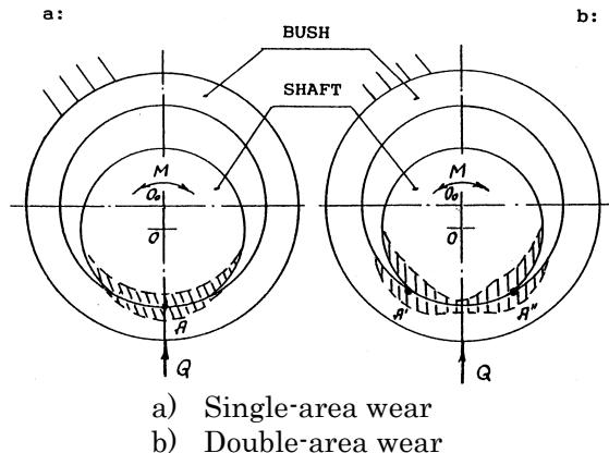
Fig.3 Projection diagram of wear
