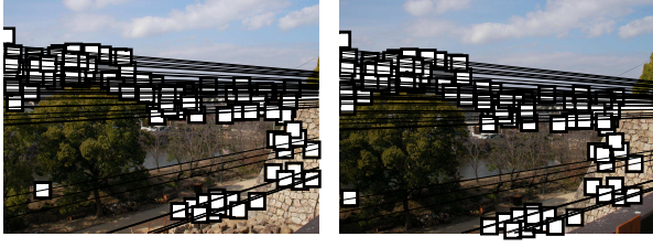
Figure 4: Corresponding points in real images and computed epipolar lines.
