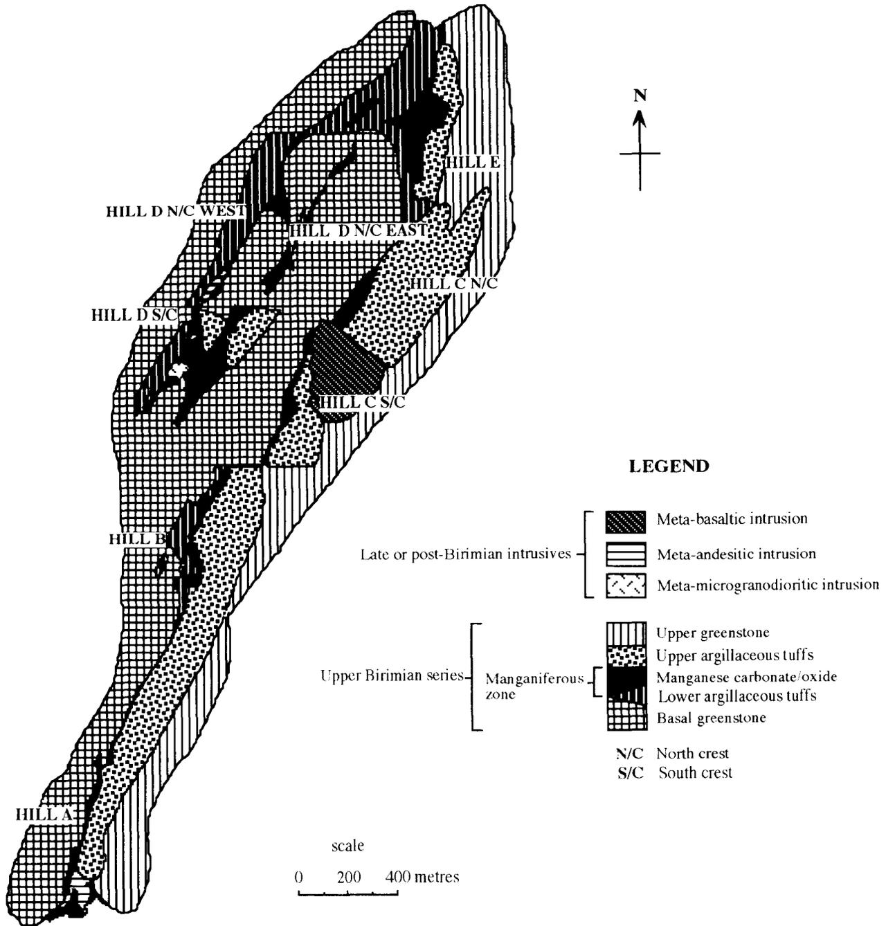
Fig. 2 Geological map of Nsuta mine area. (modified from Service, 1943)
