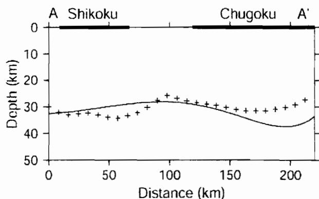
**Fig. 8.** Cross section along A-A' line of the two-dimensional variation of the Moho depth. Cross and solid curve indicate the Moho depth estimated by the gravitational and seismological methods, respectively. Location of A-A' line is shown in Fig. 3.
