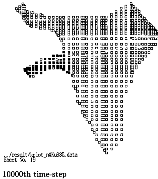
Figure 5: Unstable result by the 'ordinary' FEM in Case 2
