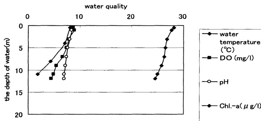
Figure 5 Water quality profiles at Point D (July 18th, 2004)
