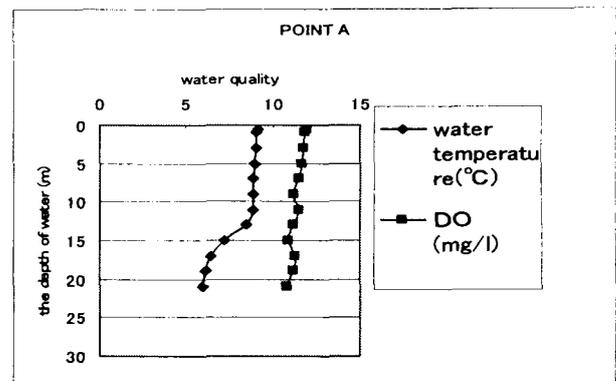
Figure 2 Water quality profiles at Point A on March 27th, 2004
