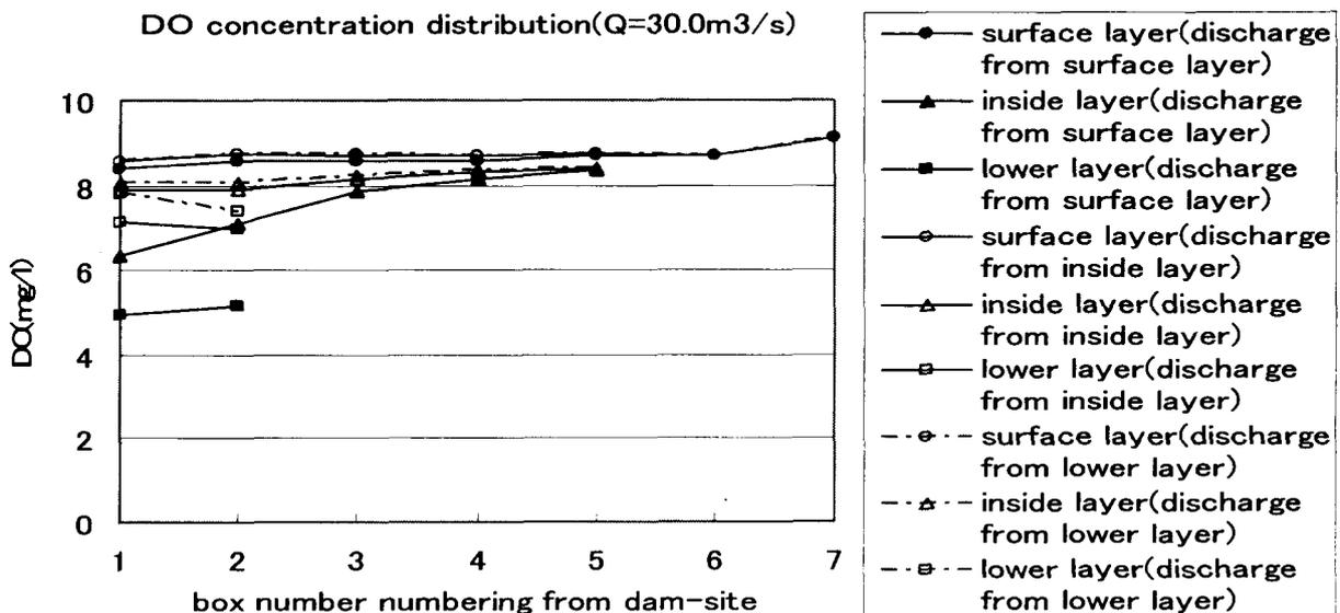
Figure 9 Calculation results for DO
