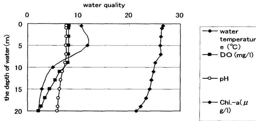
Figure 4 Water quality profiles at Point A (July 18th, 2004)
