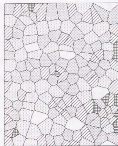
Fig.5.31 Distribution of damage \Omega_{22} for Model C_2
